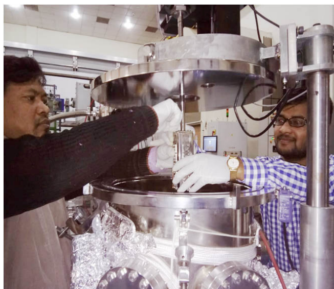
Mounting the sample ladder/holder mounted in the chamber
