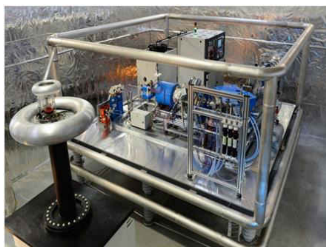
High Voltage Deck of 300 kV potential
