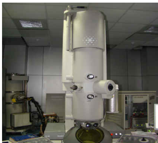
Digital Photograph of Transmission electron microscope: High Voltage Deck of 300 kV potential 300 keV TEM FEI Tecnai
